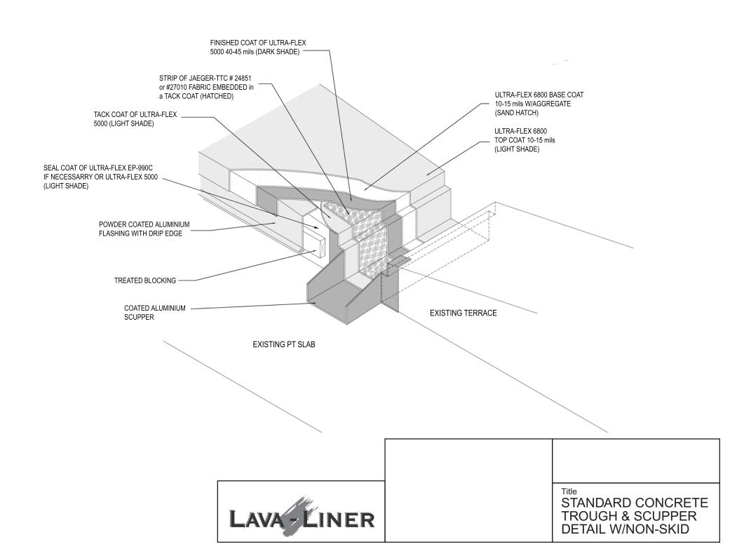
GENERAL NOTE: PRESSURE WASH EXISTING SLAB PRIOR TO INSTALLATION OF WATERPROOFING SYSTEM
